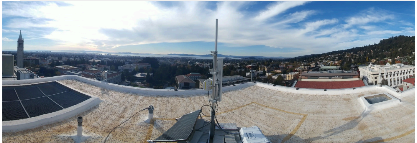
A SFWEM solar powered hub node atop Evans Hall on the UC Berkeley campus
