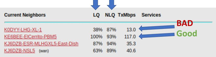
Radios automatically negotiate best modulation rate based on SNR
