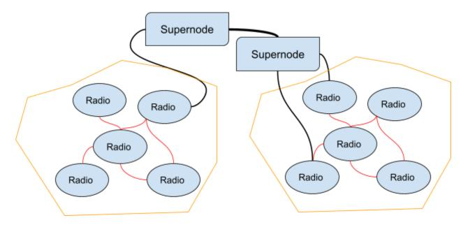
Supernodes do not merge networks into one big mesh (<u>AREDN cloud tunnel server</u>) but instead provide connections between discrete meshes.
